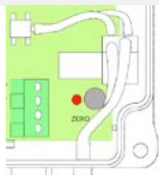
Auto zero element makes the DPT FLOW meter maintenance free. Element automatically adjusts the transmitters zero point from time to time, this eliminates the zero point long term drift of the piezoresistive sensing element.
