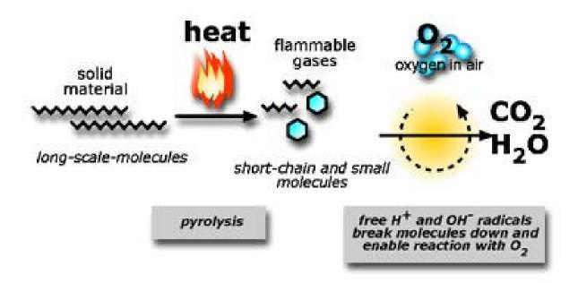
The gas flame itself is maintained by the action of high energy "radicals" (that is H\_ and OH\_ in the gas phase) which decompose molecules to give free carbon which can react with oxygen in air to "burn" to CO2, generating heat energy.
